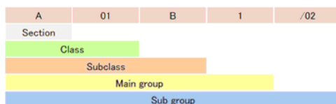
Fig. 1. A is a section for ‘Human Necessities’, A01 is class representing ‘Agriculture; Forestry; Hunting; Fishing; etc.’, A01B is subclass which consists of ‘Soil working in agriculture or forestry etc.’, A01B 1/00 is a main group representing ‘Hand Tools’, while A01B 1/02 is a subgroup for ‘Spades; Shovels’.
